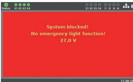
Fig. 25: Emergency lighting blocking display
