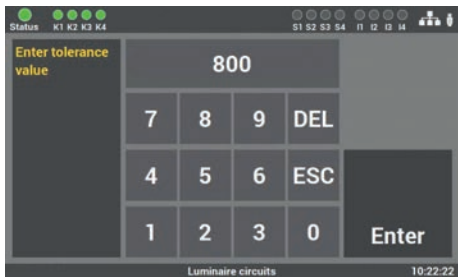
Fig. 87: Mask „Threshold values“ (electrical circuit monitoring)
